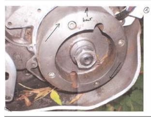
Pull the stock rotor off, you will need a puller for this. Unscrew the old stator and take it off the engine.
