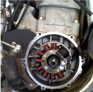
Unscrew the stator coil from the base plate and lift it a little away from it so that you can access the mounting holes. Take care not to damage the paint insulation of the coil. Put the base plate with the stator hanging loosely from the unit into the place of your old generator. Fasten the plate with the 3 screws M5x12. Take care to not jam any wires under the plate.
