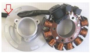
Have a look at the new stator. You will find a little left of the cable exit a small red marking. That is an ignition marking.
