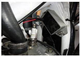
Fasten the electronic regulator in a convenient spot on the frame.
