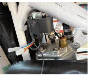
Fasten the ignition coil on the frame of the motorcycle, best there, where the original coil was.
